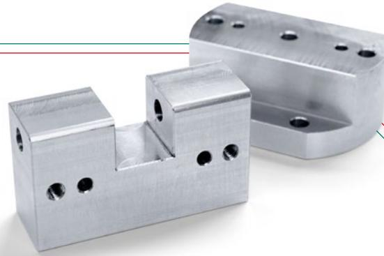
The company uses the CMX 600 V among other machines to mill mounting brackets for a welding robot and folding brackets for tandem welding units.
