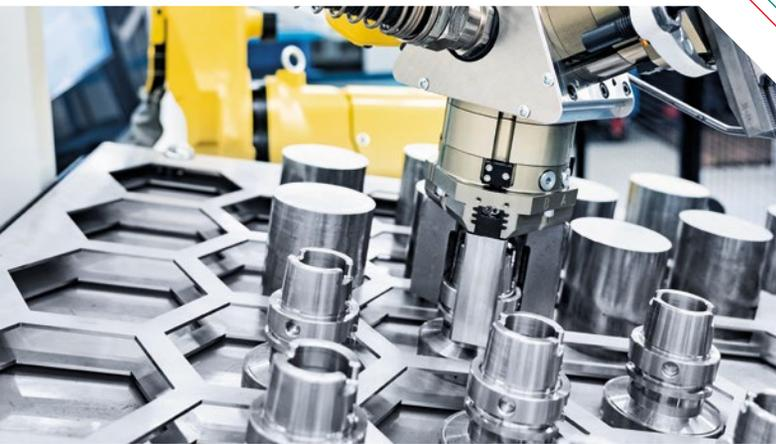
For different diameters, the Robo2Go automatically calculates the midpoint of the workpieces in order to grip them precisely.
