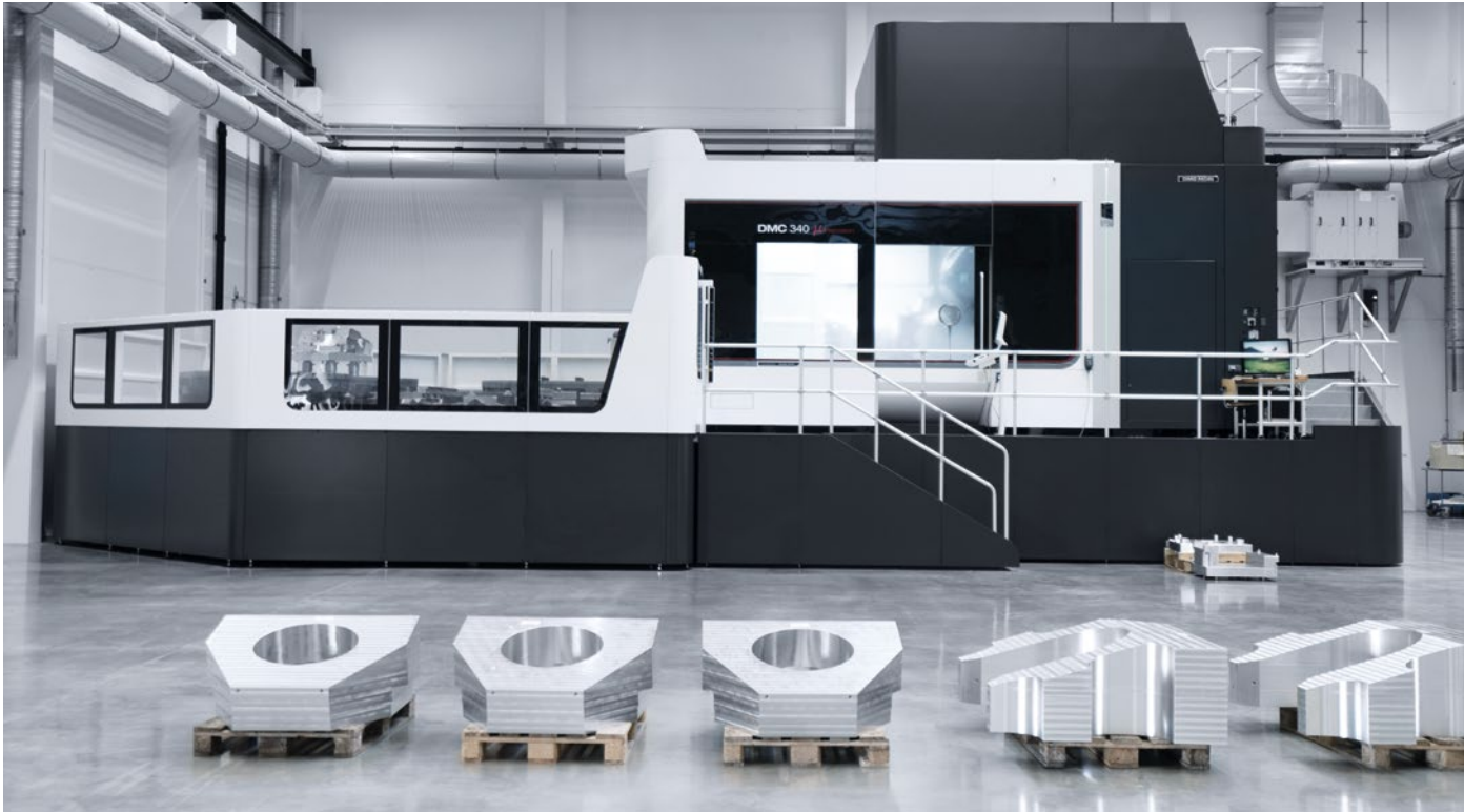
On the DMC 210 and 340 U \mu Precision, Kapplercnc manufactures high-precision components which are used in the semiconductor industry for manufacturing wafers, for example.
