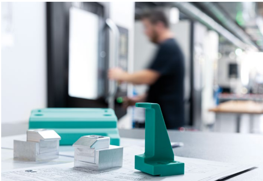
Ultraschall Technologie produces simple moldings for workholding in the ULTRASONIC welding systems. They are made of plastic and titanium, among other materials.
