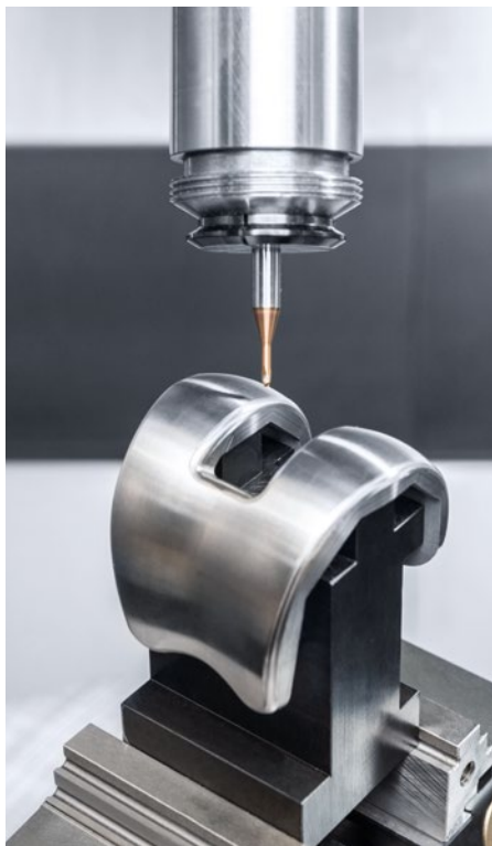
The Fraunhofer IPT also tests its software on workpieces from other sectors – here on a knee implant.
